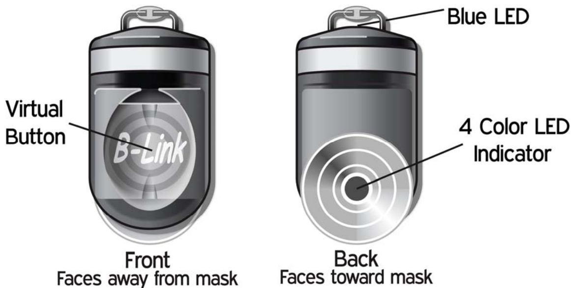
FIGURE 2. Tapping the virtual Button on your B-Link causes the LEDs on your Buddy’s unit to flash and a tone to sound.
