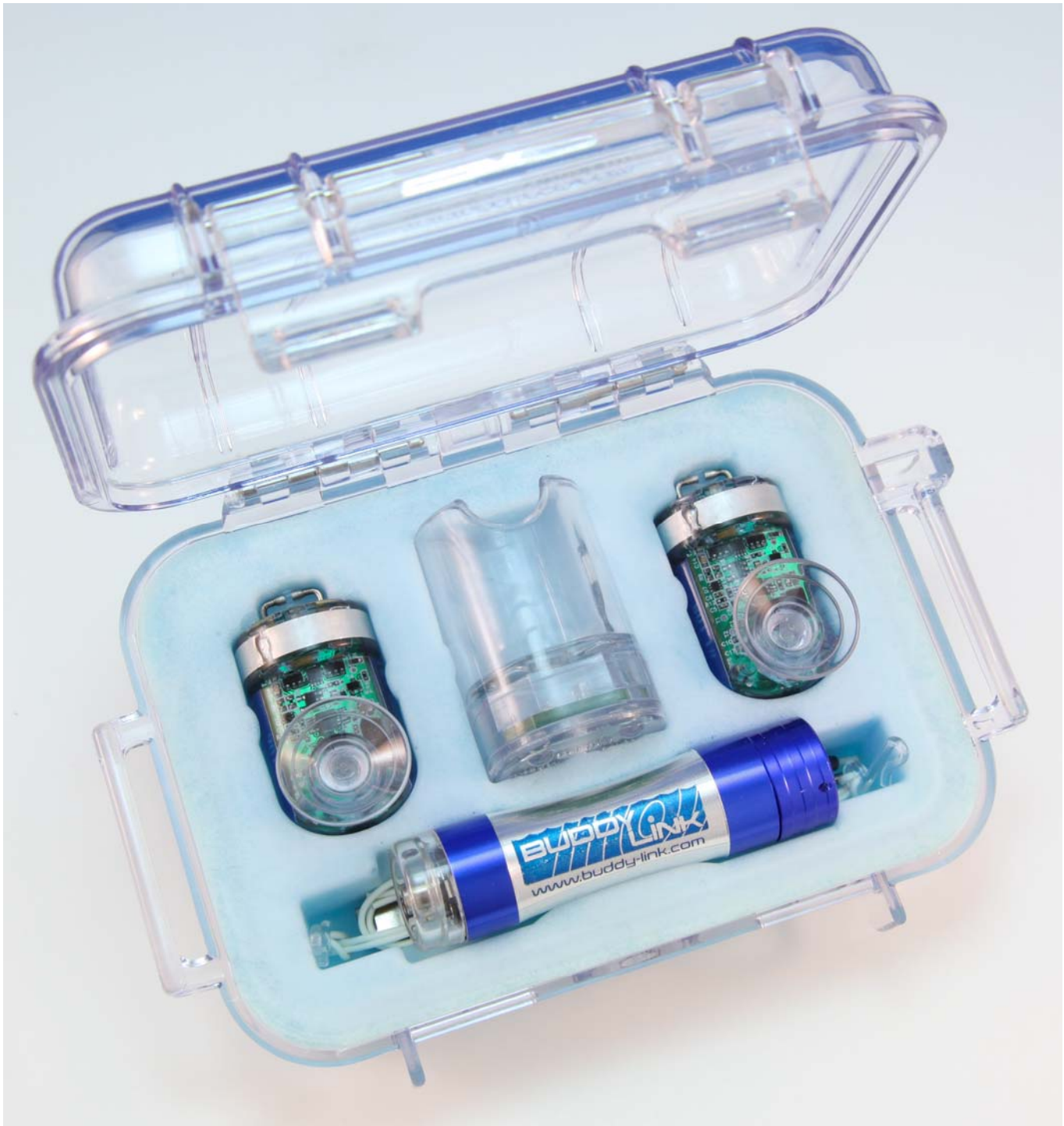
FIGURE 13. B-Links are delivered in a water-resistant Pelican case with molded polyurethane foam liner, and includes 2 B-Link units, 2 Lanyards, a Charging Station, a DC-to-DC Converter, and a connecting cable.
