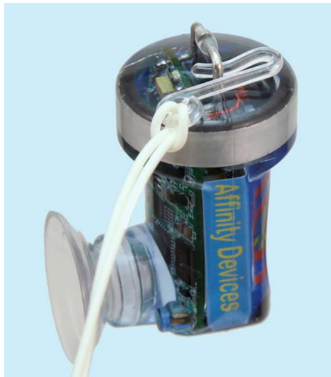
FIGURE 3. Hook the plastic Lanyard Clip on the B-Link's stainless steel terminals, and attach the safety Lanyard to the mask strap.
